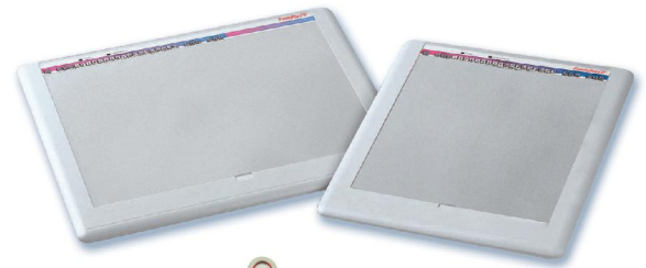
DrawingBoard VI digitizers work with a variety of cursors and stylus pens
